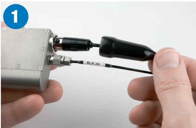
Pull the sleeve back, align the pins on the plug and jack and insert the connector.
