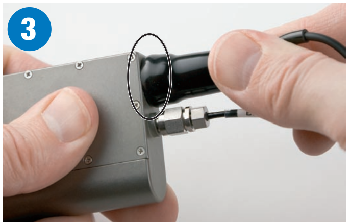
When the sleeve is completely seated, it will sit flush against the housing with the inside of the sleeve gripping the flange all the way around the connector.
