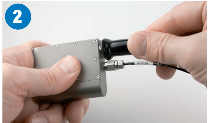
Pinch and push the sleeve over the flange on the connector. It helps to pinch the sleeve close to the housing to work the edge over the flange.
